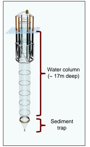
• 9 mesocosms (made of 1 mm thick thermoplastic polyurethane, 2 m diameter) containing a natural phytoplankton community
