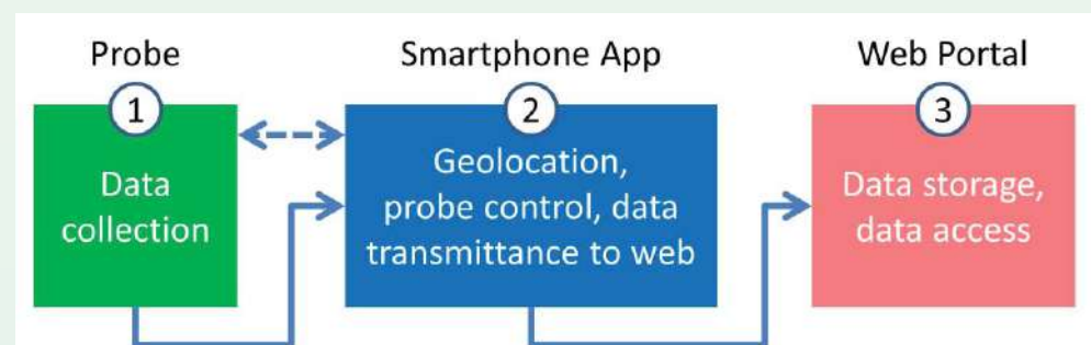
Fig. 1: Suggested system for temperature profiles collection.
